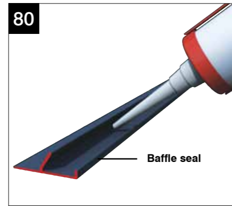
80 An aluminium extrusion is provided to give an additional seal at the ridge. Silicone seal along the length of the 'V' slot.
