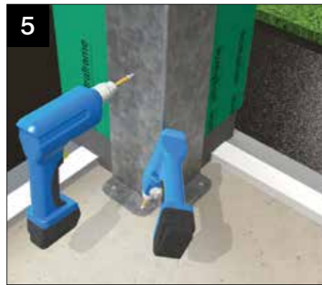
5 Lift column into place and fix to the structural bracket using fixings from SLP005 kit. Ensure that the tall columns are positioned to the front of the structure. Repeat steps 3, 4 and 5 for each of the four columns.
