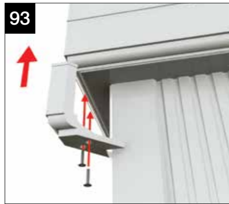
Whilst ensuring that the corner remains located in position, screw fix using self drilling screws CRN007.
