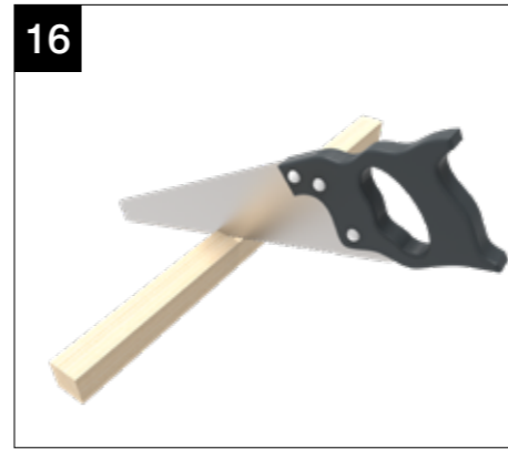
16 Cut the 45 x 45mm battens to length, these should be cut to the same length as the external walling clips.
