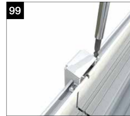
Whilst ensuring the in-line joint remains in position, screw fix using CRN007.
