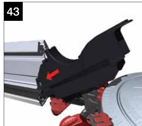
Next, attach the speedlock hood over each bar, sliding it under the co-extruded gasket of the glazing bar undercladding.
