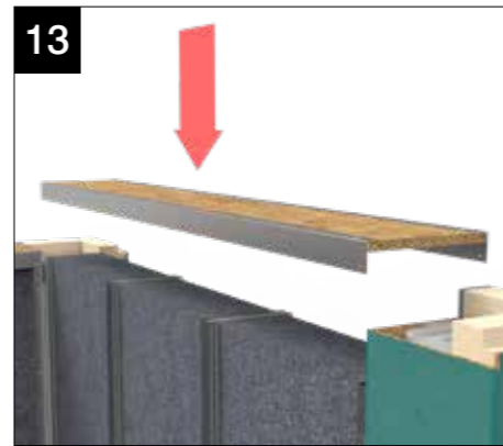
13 Position the walling top tray on the walls so that the internal steel flange is against the walling clips. It may help at this stage to secure the top tray to the column by diagonally fixing into the column through the OSB tray pulling the two components together.
