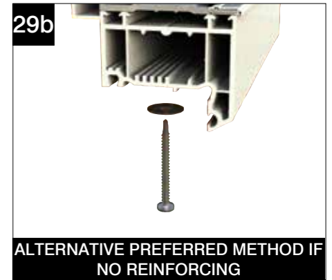
Behind the head of the screw, use a 20mm washer so that the thread is biting into the aluminium eaves beam. NOTE: Trim back any screw points protruding through the eaves beam to make flush.
