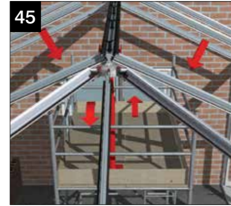
Continue to attach all the glazing bars using the location plan provided to check each bars final position with its corresponding label.
