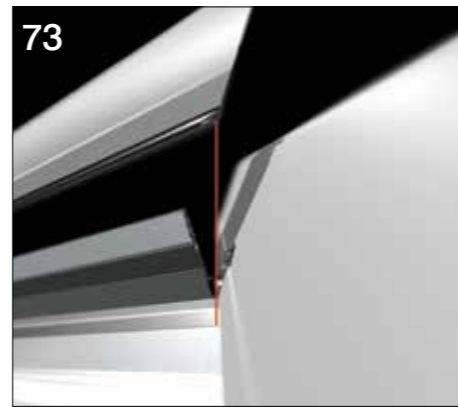
73 Ensure the jack rafter top capping is lined up correctly (as above) before knocking the top cappings into position.
