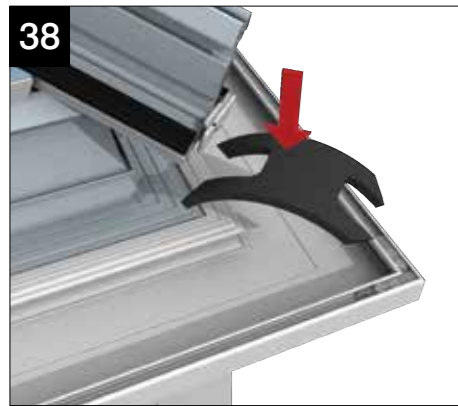
At 90° corner insert 'H' section and press down. Similarly apply at stop end or outlet positions.
