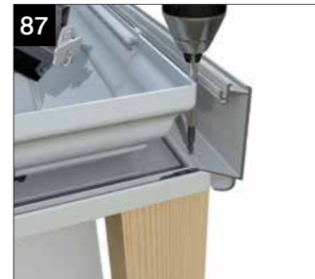
87 Offer up the middle cornice section into position, (it may be advisable to temporarily support the lower cornice section whilst fixing) secure using fixings provided (CRN007). (Long reach driver required).
