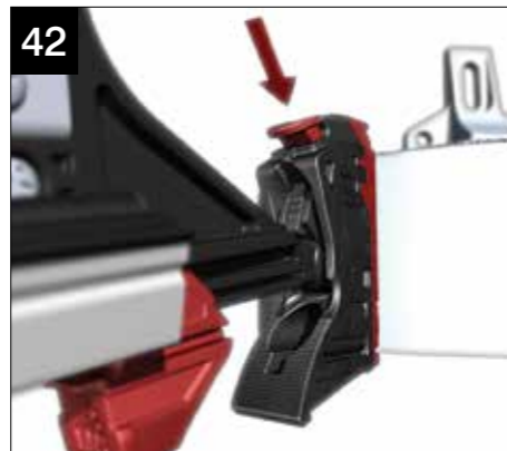
Attach bar at eaves position. Using your thumb push down the upper dead lock so it's flush. YOU MUST NOT PUSH UP THE LOWER WEDGE LOCK YET. To remove the bar, lever up the dead lock using a flat blade screwdriver, then insert the screwdriver to release the socket latch.
