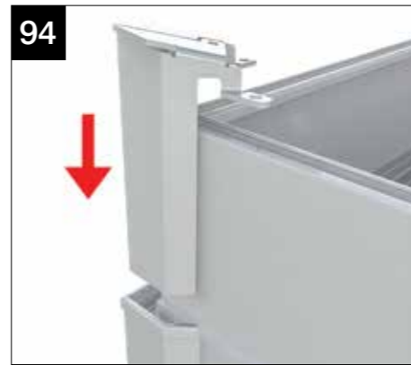
Slide down LANC090 so bracket cleats slot into top section.
