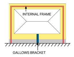
All box beams that support a 265mm fabricated box gutter must be supported by means of gallows brackets, posts or brick piers. Min/max. dimensions from internal frame stated below.
