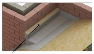
47.5mm packed off timber has been used to pack off the box gutter to line up with the standard gutter.
