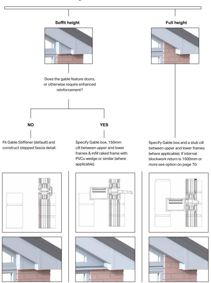
Note: when Gable box is present, notching will be required to internal blockwork to accommodate.
