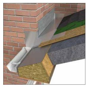
**A tapered box gutter** is used in this situation, it fits normally and flush with the host wall and roof.
