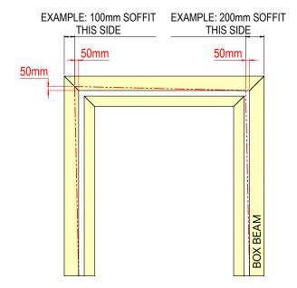
The deviation that is possible on standard 40mm soffit without on site modifications to parts is 10mm.
