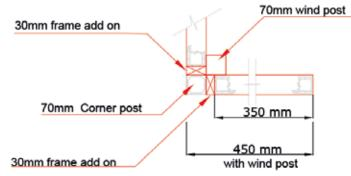
Minimum Frame Return Detail with wind post (When adjacent/in line with 4m unsupported span)
