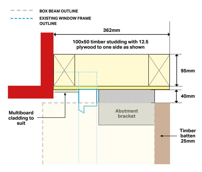
Replace existing frame with 100x50 (MIN) timber studding with 12.5mm plywood to bracket, fixed back to host wall and floor or dwarf wall.
