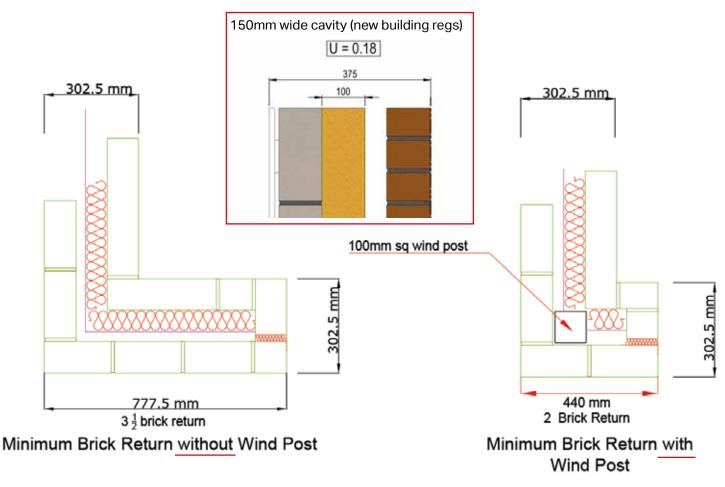
(When adjacent/in line with 4m unsupported span)
