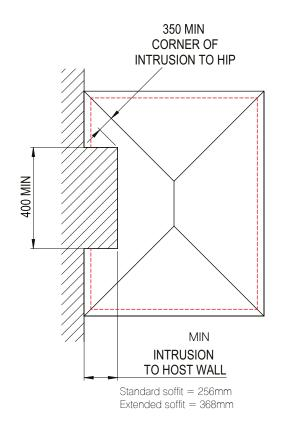
No glazing allowed in roof sections where there is an intrusion
