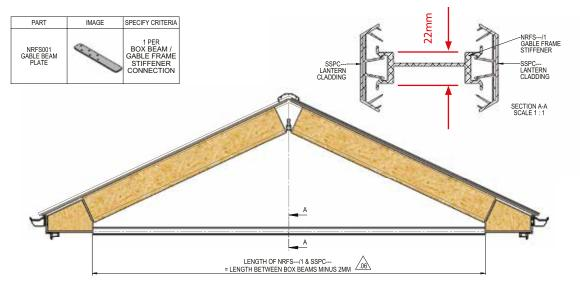
**All gable frame sizes are provided as tight sizes.** You will need to adjust your gable frame size slightly to give you clearance between the underside of the roof and the gable frame to aid installation.
