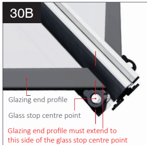
30B If positioned correctly the glazing end profile will extend beyond the centre point of the glass stop.
