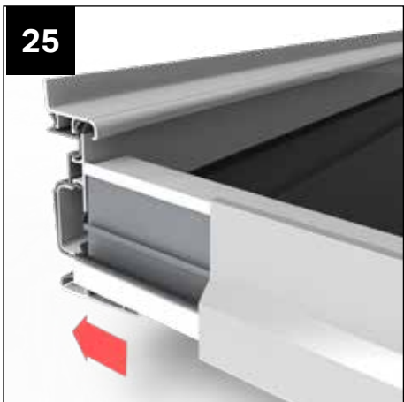
Apply silicone to the gable side cappings and fit to the gable bars. These may require cutting in for a low pitch ridge. TIP: Screw the side capping to the gable bar at the top and bottom where the screw will be covered by the end caps.
