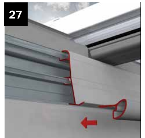
Push fit the internal fascia trim into position.
